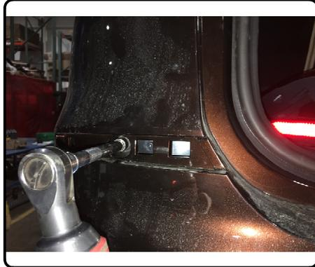
11. Remove bumper beam by removing (2) nuts on each side using 18mm socket. Also remove (1) nut on each side from exhaust hanger that is attached to bumper beam using 13mm socket. Remove passenger side hanger and return to owner. If present, unclip electrical harness.
