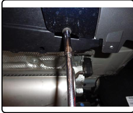
2. Located on bottom of rear fascia remove (3) fasteners on each side using 8mm socket. Inside wheel well trim remove (1) fastener on each side using 8mm socket
