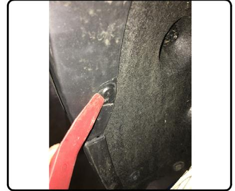
4. Remove (2) fasteners from each side of bumper cover using 8 mm socket which are now accessible due to wheel well trim removal.
