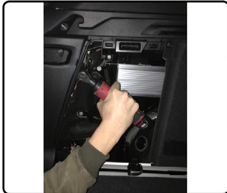
7. Remove (2) nuts from each tail light using 10mm socket.
