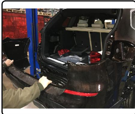
12. Raise hitch and bumper beam into position onto vehicle studs and secure using existing vehicle hardware. Use vehicle hardware to reattach driver side hanger bracket. Use hanger on hitch to reattach passenger side exhaust. **NOTE:** Remove driver side exhaust bracket stud and replace with provided M8 hardware.
