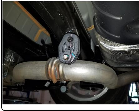
4. Locate and remove (2) plastic nuts with a 10mm socket. Remove heat shield and mark out a 5" x 13" section with masking tape. Use aviation shears to trim marked area. Reinstall with (1) nut using a 10mm socket.
