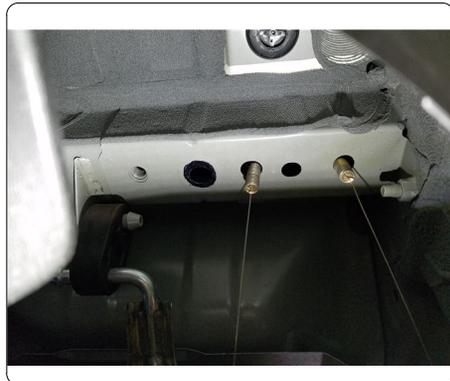
5. Raise hitch into position feeding the (2) fishwires through the rearmost holes on hitch. Remove fishwires and use (3) M12 bolts from step 2, (1) M12 bolt and (1) 1/2" conical tooth washer, and (2) 1/2" hex flanged nuts to fasten hitch to vehicle.
