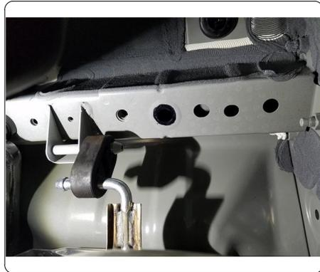
4. Fishwire (2) 1/2" carriage bolts and (2) CM-SP12 spacers through the access hole in the driver side frame rail.
