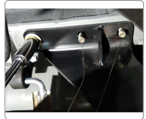
6. Torque M12 hardware to 79 ft-lbs. and 1/2" hardware to 110 ft-lbs.
