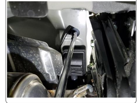
2. On the passenger side, remove (6) M12 bolts using an 18mm socket, to remove tow loop. Return tow loop to vehicle owner. Reinstall emissions canister following step 1 in reverse order.
