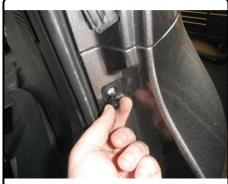
5. Remove (1) screw per each side of vehicle inside of rear wheel well that are attaching the rear fascia to the vehicle side panels.
