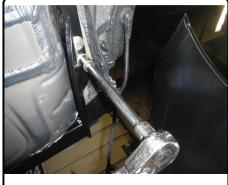
9. Raise exhaust back into position. Reinstall rear fascia in reverse order of removal from Steps 4-7.
