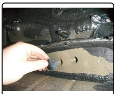
4. Open rear hatch of vehicle and remove (1) plastic rivet and (2) screws per each side of vehicle that are attaching the rear fascia.
