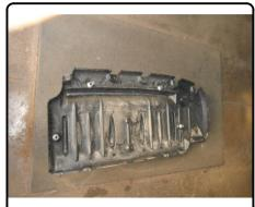
2. Lower exhaust by disconnecting (1) rubber isolator. (See Rubber Isolator Removal Diagram)
