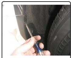
6. Remove (2) plastic clips on passenger side and (1) on driver side at bottom edge of fascia near wheel well.
