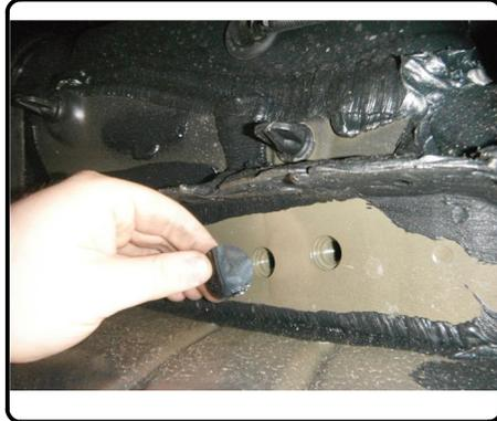
4. Open rear hatch of vehicle and remove (1) plastic rivet and (2) screws per each side of vehicle that are attaching the rear fascia.
