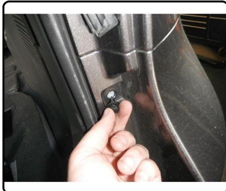
5. Remove (1) screw per each side of vehicle inside of rear wheel well that are attaching the rear fascia to the vehicle side panels.
