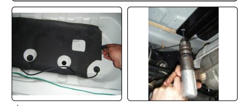
7. Install 1/2-13 x 1 3/4" carriage bolts and SP6 spacers in the rear-most holes of trunk pan. Install 1/2-13 x 1 3/4" carriage bolts and SP4 spacers in the forward-most drilled holes of trunk pan. Secure bolts using 1/2-13 flange nuts. Use silicone caulk or equivalent to seal holes in trunk. Re-install carpet, foam spare tire locator, and spare tire.
