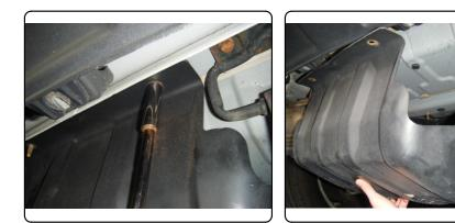
3. If needed bend back heat shields and remove (4) M10 nuts from the bumper bracket weld studs.
