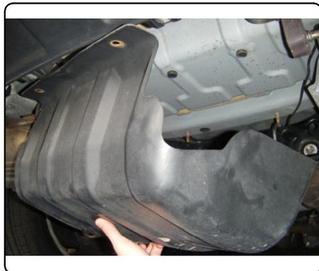
3. If needed bend back heat shields and remove (4) M10 nuts from the bumper bracket weld studs.
