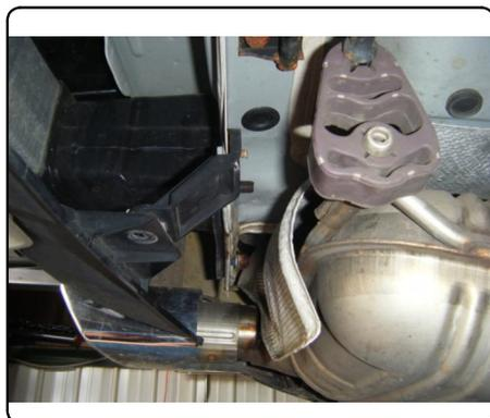
4. Raise hitch into position and secure to bumper bracket weld studs using (4) M10 nuts removed in Step (3). Re-install (2) fascia screws removed in Step (1). **Note:** Gently flex fascia and fascia brackets to slide hitch into position. You may temporarily remove (2) fascia brackets if needed.
