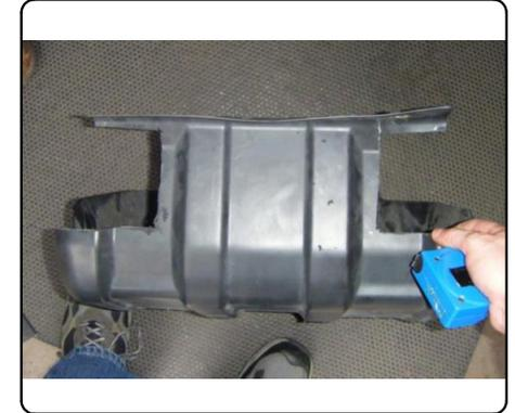
9. Bend heat shields back into original position. Hitch install is complete.
