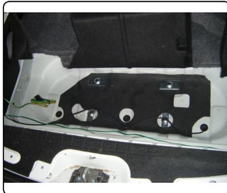
8. Torque all M10 fasteners to 48 ft-lbs. Torque all 1/2" fasteners to 110 ft-lbs. If desired you may trim the trunk pan cover and re-attach using nuts removed in Step (2). **Note:** Dimensions are approximate, confirm fit prior to trimming.
