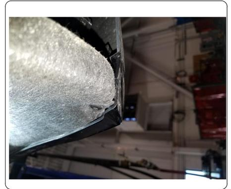
2. Pull away wheel well lining to reveal (6) screws, (3) on each side, and remove using a T25 torxbit socket.
