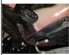
Remove (3) plastic push pins and (2) plastic nuts securing the plastic panel using a screwdriver and a 14mm socket. Mark out a 3" x 5" section using masking tape and trim using aviation shears. Confirm trim prior to reinstallation.
