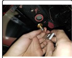
4. Raise hitch into position and feed fishwires through center hole on the hitch. Remove fishwires and loosely secure with 7/16" hex flange nuts.
