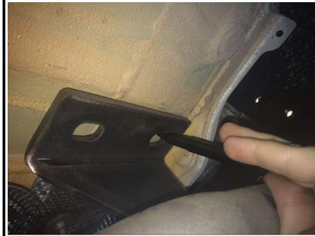
4. Lower the hitch and use a drill and 5/16" drill bit to drill (5) holes located at the marked areas from step 3. Then use 9/16" drill bit to open up the holes to the final size.
