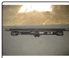
4. With the hitch side plates flat on the ground, align the center holes of the hitch with the bolts fishwired in the bumper beam and loosely secure with 1/2" flange nuts. Raise the hitch and bumper beam into position by aligning the hitch and bumper beam holes with the holes in the end of the frame. Secure with the M10-1.25 x 30mm hex flange bolts provided and the M10 nuts removed in Step (2).
