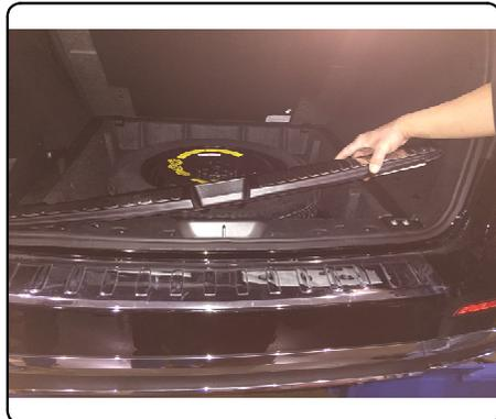
5. Inside trunk locate and remove bumper beam nuts, (2) on each side, using 16mm socket.
