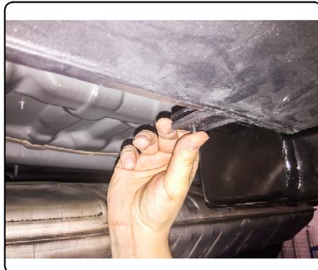
9. Torque all 1/4" hardware to 10 ft-lbs and all M10 hardware to 45 ft-lbs. Reinstall following steps 2 - 4 in reverse order.
