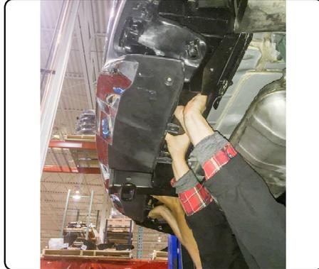
8. Secure provided fascia tab brackets to hitch main body plates, with 1/4" hardware, using 7/16 socket and 7/16" boxed end wrench. Align and secure (2) center fascia tabs by pushing nylon retainer clips into fascia tab brackets.
