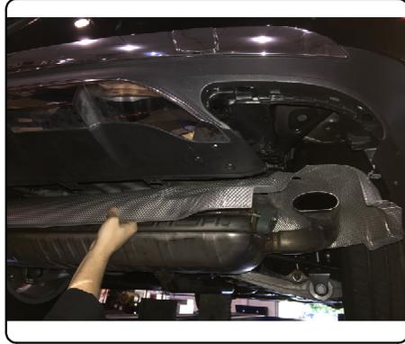
4. Remove trunk liner guard using T-30 socket to remove screw. Gently unclip trunk liner guard and remove trunk contents to expose bumper beam nut inside vehicle. Set aside trunk contents and trunk liner guard for reinstallation.
