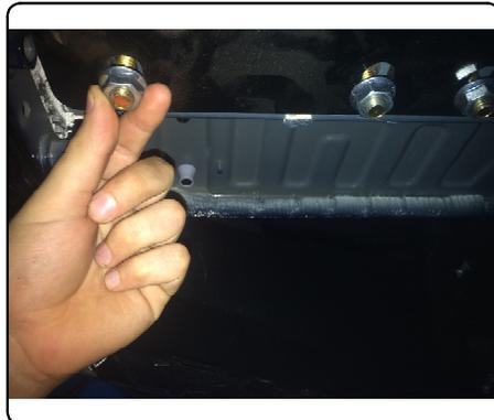
5. Use an 11/16" socket and torque all 7/16" hardware to 59 ft-lbs. Raise exhaust back into position and reinstall rubber isolators removed in Step 1.
