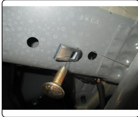
4. Gently pull fascia down and raise hitch into position guiding fishwires through mounting holes. Leave fishwires attached. NOTE: Hardware may need to be temporarily pushed into frame to position hitch over bumper beam studs. Remove fishwires & loosely secure 7/16 nuts. Secure existing M10 nuts onto bumper beam studs.
