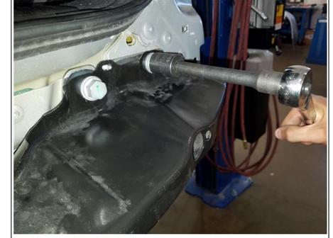
6. Raise hitch into position lining up the holes with the hole in the bumper beam and loosely fastening the (8) M14 bolts removed from Step 5. Torque the M14 bolts to 126 ft-lbs. Reinstall following steps 1-5 in reverse order.
