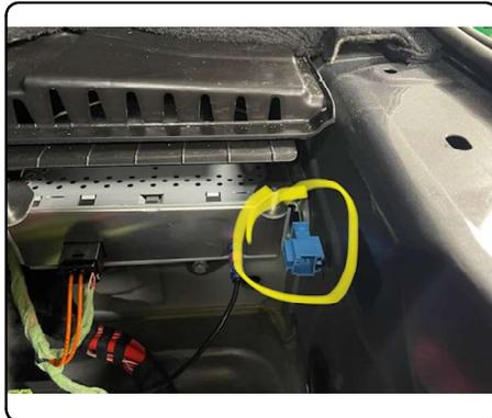
3. Remove lower rear fascia by locating and removing (6) screws (3) on each side using 10mm socket and (4) push pins (2) on each side using pry tool. Unclip electrical harnesses.
