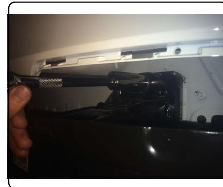
8. Reinstall exhaust bracket if removed in step 5. Reinstall trimmed heat shield removed in step 4. Reinstall lower rear fascia removed in step 3. Raise exhaust back in position. Reinstall exhaust tips removed in step 1. Reinstall all hardware removed. Reinstall items removed in step 2A and 2B.
