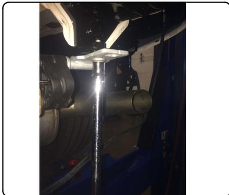
6. Install hitch on rear of vehicle frame using existing studs. Reinstall bumper beam over hitch. Loosely secure M12 hardware.
