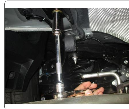
6. Torque all 1/2" fasteners to 110 ft-lbs. Raise exhaust back into position and re-install exhaust hangers.
