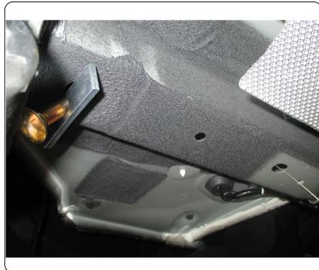
4. Reverse fishwire one (1) 1/2" carriage bolt and one (1) CM-SP6 through access hole in each frame rail. Leave fishwires attached.
