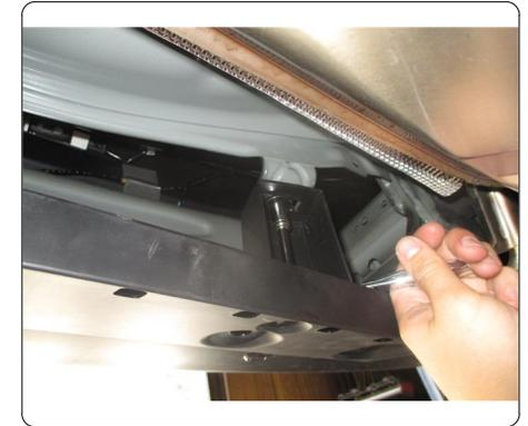
2. Remove four (4) rubber exhaust hangers using exhaust removal pliers or method shown above. Make sure exhaust is supported.
