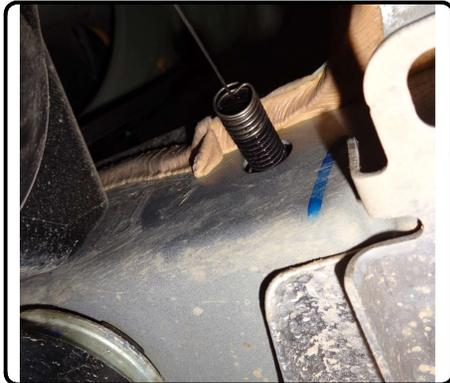
5. Raise the hitch into position, thread the fishwires into the mounting holes. On the bottom attachments, place a CM-SP10 spacer on the bolt and loosely install all 1/2" hex flange nuts with a 3/4" socket.
