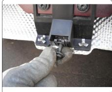
b. ON V60, V70 AND XC70 MODELS ONLY Open hatch. Remove two rubber hatch stops. (See Figure 2)
