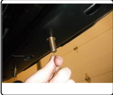
2. Raise hitch into position between bumper mount plates and align slots in hitch with existing vehicle weldnuts in the frame rails. Install (4) M12-1.25 hex bolts and (4) 1/2" conical toothed washers into existing weldnuts, as shown.
