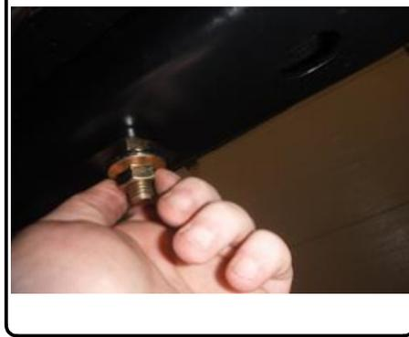
3. ROTATE BOLT AND SPACER THROUGH MOUNTING HOLE
