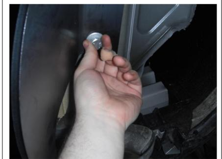
6. Torque 1/2" hardware to 110 lb-ft and M12 hardware to 79 lb-ft.
