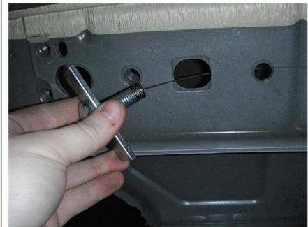
5. Raise hitch into position by placing passenger side of hitch over the passenger side muffler first and then raise the driver side of hitch. Secure hitch to existing weldnuts with supplied M12 hardware and conical toothed washers. Attach 1/2" hex flange nuts onto carriage bolts.
