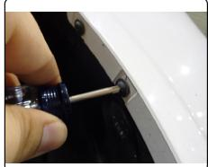
2. Remove (2) fasteners located at the top of the bumper cover hidden behind the wheel well with a T27 socket.
