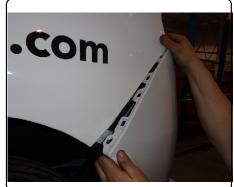
5. Disconnect the harness at the bumper. Then, place the bumper cover aside. Remove (6) bolts for the bumper with a 15mm socket, and set the bumper aside.
