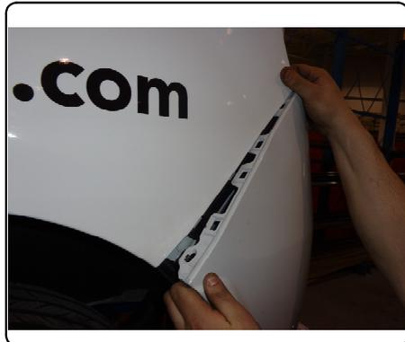
5. Disconnect the harness at the bumper. Then, place the bumper cover aside. Remove (6) bolts for the bumper with a 15mm socket, and set the bumper aside.
