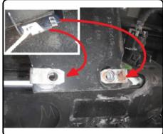
2.) Remove (4) bolts securing the factory cross member or hitch to the frame rail with a 21mm socket. Set hardware aside for reuse during CURT hitch installation. Note: The bumper shares the same mounting points and should be supported from underneath.
