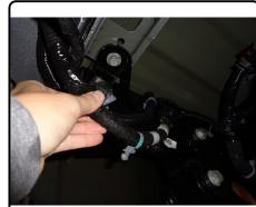
4.) Using the existing mounting hardware, attach the bottom mounting bolts (2 places each side) and loosely secure so that bumper placement adjustments can be made. Adjust bumper position to align with side mounting holes and secure remaining (4) bolts with a 21mm socket.
