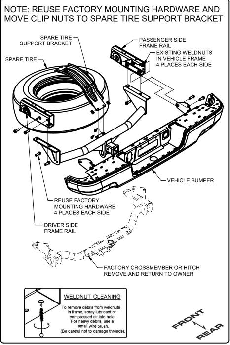
1.) Lower spare tire using the vehicle service tools located in the cab of the truck. Loosen the spare tire support bracket by removing (2) bolts with a 13mm socket by the spare winch. Remove the 2 bolts from the factory hitch or cross member and transfer the (2) clip nuts onto the spare tire support bracket.
