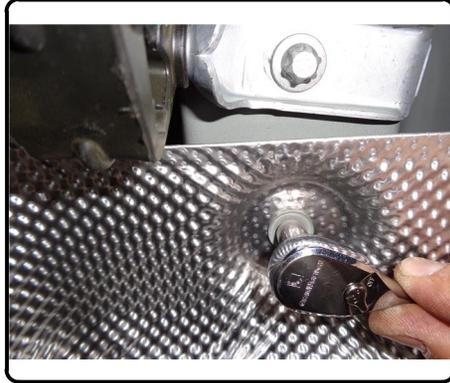
13) Trim heat shield with shears around lower portion of hitch to avoid any contact. Approx. dimensions of cut out should be 1.25" x 4.50".
