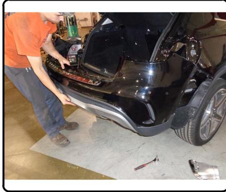
8) Remove (8) M10 nuts on inner panel to remove the bumper, (4) per side. Remove bumper. Set aside bumper and hardware for reassembly.
