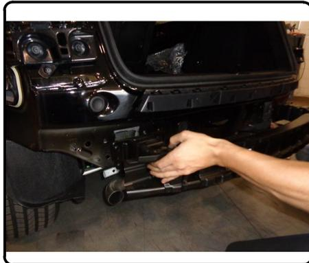
9) Align hitch on bumper through the weld on bolts.
