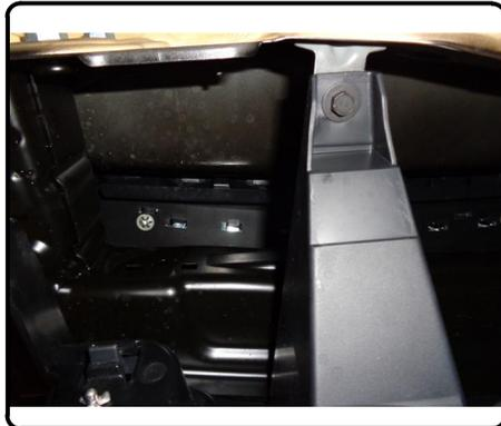
5) Remove (6) M6 bolts from exhaust heat shield. Do not remove heat shield, leave in place. Lower and lay on exhaust.
