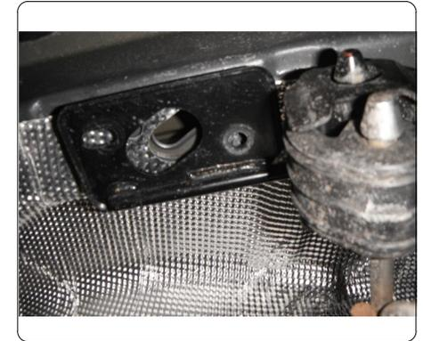
2. Enlarge the access hole to allow 7/16" carriage bolts to pass through on both vehicle frame rails.
