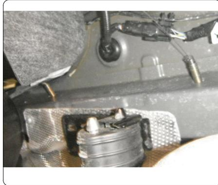
4. Slide the hitch in from the rear passenger side of the vehicle over the exhaust and into position. Secure hitch to side plates with 7/16" carriage bolts and loosely install 7/16" flange nuts as shown below.
