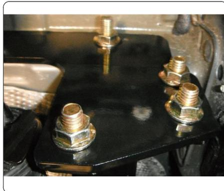
5. Reattach the muffler brackets removed in step 1. Torque to 16 ft-lbs.
