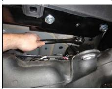
9. Raise mounting strap (B) into position and loosely secure to hitch 1/2-13 x 1" carriage bolts and 1/2-13 hex flange nuts. Raise nut plate (C) into position and secure mounting strap to the cross member using 1/2-13 x 3" hex bolts and 1/2" conical toothed washers. Torque the 1/2-13 x 3" hex bolts to 75 ft-lbs.
