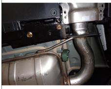
8. Center the holes of the hitch with the bumper beam tab weldnuts and secure with M8 bolts. Torque all M8 fasteners to 25 ft-lbs.
