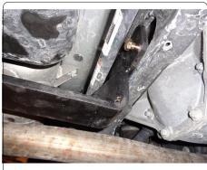
Secure the (2) center fascia tabs by pushing the nylon retainer clips into the holes in hitch tube.
