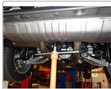
3. Disconnect heat shield bolts for trimming and hardware access. Remove (1) bolt from each side near the frame flange with an 8mm socket.
