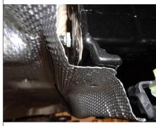
4. Trimming: Use shears or rotary cut-off wheel Heat shield: Trim approx. 11" x 6" area as shown following the curvature of the heat shield.
