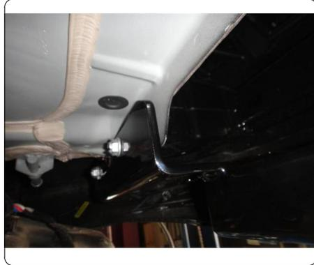
7. Stack bolt plate (D) on spacer plate (E) and run 1/2-13 x 1 1/2" carriage bolts through plate holes. Place plate assembly over the bumper beam tab and align with the holes in the hitch. Secure using 1/2-13 flange nuts, as shown.
