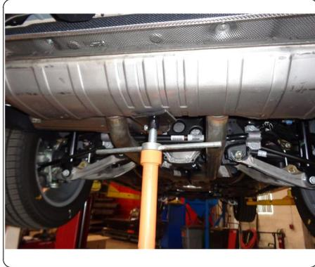
3. Disconnect heat shield bolts for trimming and hardware access. Remove (1) bolt from each side near the frame flange with an 8mm socket.
