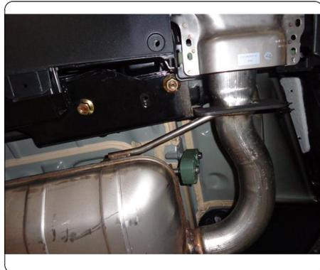
8. Center the holes of the hitch with the bumper beam tab weldnuts and secure with M8 bolts. Torque all M8 fasteners to 25 ft-lbs.
