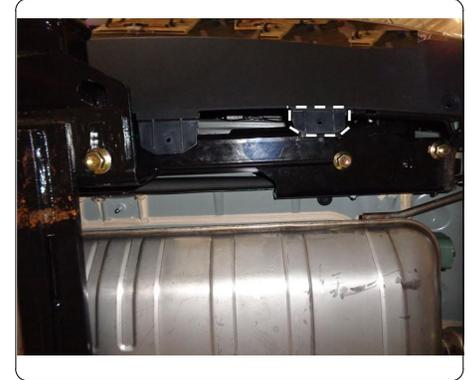
5. Remove the lower (2) nuts securing the bumper beam to the vehicle with a 10mm socket, both sides. Save for reassembly.
