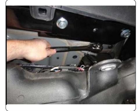
9. Raise mounting strap (B) into position and loosely secure to hitch 1/2-13 x 1" carriage bolts and 1/2-13 hex flange nuts. Raise nut plate (C) into position and secure mounting strap to the cross member using 1/2-13 x 3" hex bolts and 1/2" conical toothed washers. Torque the 1/2-13 x 3" hex bolts to 75 ft-lbs.
