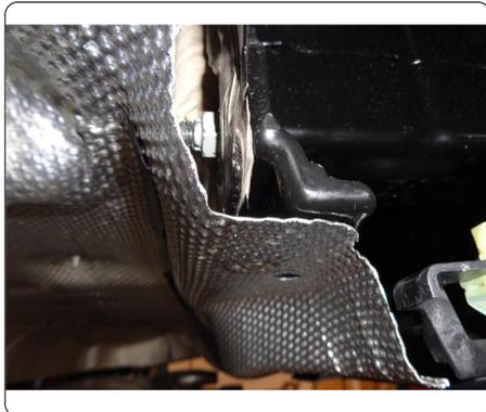
4. Trimming: Use shears or rotary cut-off wheel
