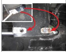
2.) Remove (4) bolts securing the factory crossmember or hitch to the frame rail with a 21mm socket. Set hardware aside for reuse during CURT hitch installation.
