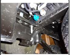
Install 1/2" carriage bolts, spacers, and flange nuts in remaining holes as shown. Torque all 1/2" hardware to 110 ft-lbs.
