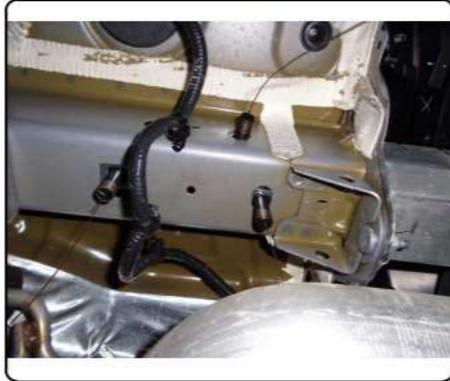
4. Raise hitch up from in front of the exhaust and into position, using care not to push hardware back inside frame. Be sure to loosely secure hitch with the mounting hardware to align all holes before tightening.
