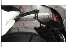
2. Lower exhaust by removing (3) rubber isolators. Support exhaust as needed to prevent damage.
