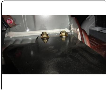
5. On the passenger side, fishwire the 1/2-13 x 4-1/2" carriage bolts through the passenger side plate and out the frame rail, secure using the 13163-SP spacer and 1/2-13 flange nuts. **Note:** If the inner bumper bolt was backed out in Step 3, tighten and torque to 25 ft-lbs.
