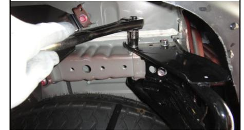
2. Lower exhaust by removing (3) rubber isolators. Support exhaust as needed to prevent damage.
