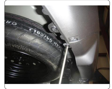
2. Raise hitch into position and secure to the existing weldnuts with M10-1.25 x 25mm bolts and 7/16" conical toothed washers. **Note:** You may need to lower spare tire for additional clearance.
