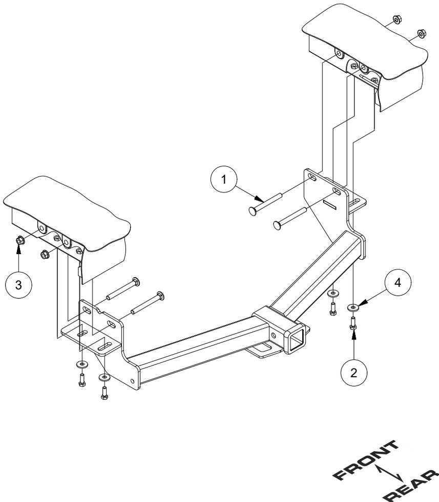
1. Remove (2) fascia screws and lower center bumper fascia panel. **Note:** Panel can be reinstalled after hitch installation is complete.
