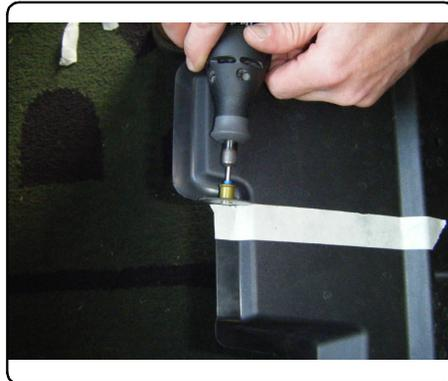
17. Raise fascia back into position, check for proper fit and clearance. If fascia doesn't fit properly trim and try again. Reattach fascia using existing hardware removed earlier. Return all unused hardware to vehicle owner.
