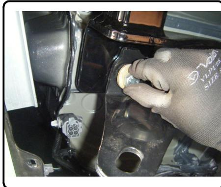
13. Torque all 12mm fasteners to 86 ft-lbs.
