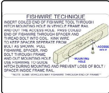
5. Locate square access cover on the outside of the bumper fascia on the passenger side of vehicle. Push in on side of cover with the arrow to open. Fishwire 7/16-14 x 1 1/4" carriage bolt and SP2 spacer through fascia access hole and out enlarged hole in passenger side bumper beam. Replace access cover when finished.
