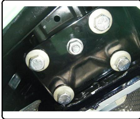
8. Insert 7/16-14 x 1" carriage bolts through top of square holes behind receiver tube of hitch. Raise mounting strap between vehicle crossmember. Loosely secure mounting strap to hitch with 7/16" flange nuts.
