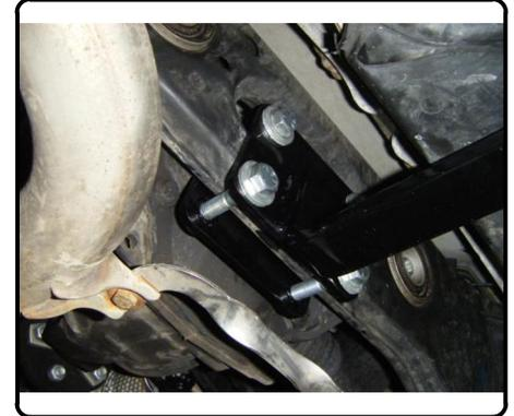
10. Torque all 1/2-13 x 5" hex bolts to 75 ft-lbs. Torque all remaining 1/2" hardware to 110 ft-lbs and all 7/16" hardware to 59 ft-lbs. Reinstall (2) screws removed in Step (2). Raise exhaust back into position. Hitch installation is complete.
