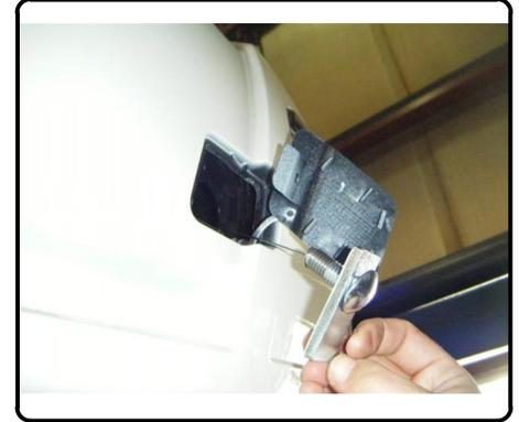
6. Place supplied nut plates over bumper beam. Raise hitch into position over exhaust and loosely secure hitch into place with 7/16" flange nuts. **Note:** Be sure to slide hitch as far forward as possible but not so it rests on the weld seam on the vehicle bumper beams.
