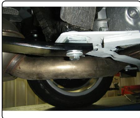
5. Torque all 12mm fasteners to 82 lb-ft, and all 7/16" fasteners to 70 lb-ft.
