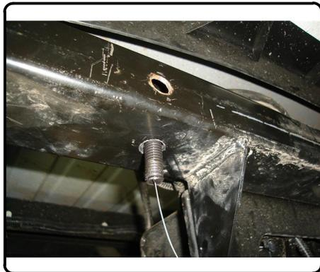
4. Raise hitch into position and install 1/2-13 X 4" lg. carriage bolts, blocks and 1/2-13 hex flange nuts loosely, as shown.
