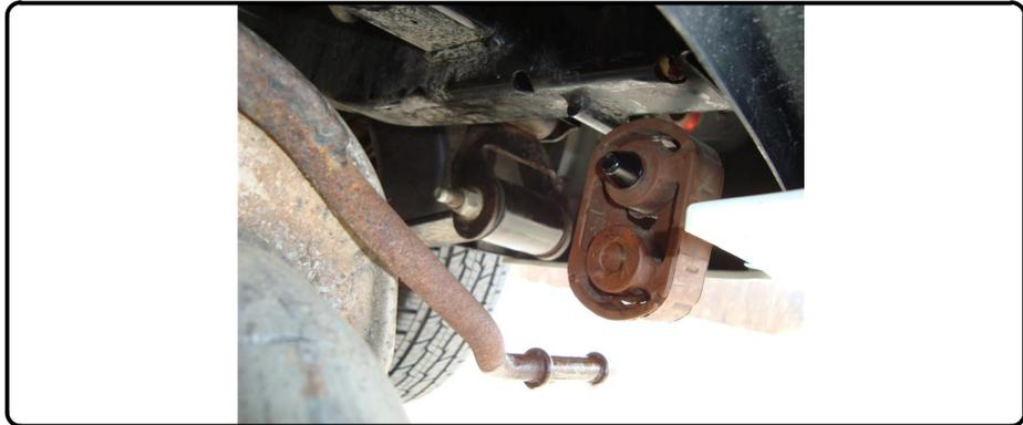
2. Locate 2 holes in vehicle crossmember, which correspond to slots in hitch side arms, and enlarge with 1/2" drill bit (See View A).
