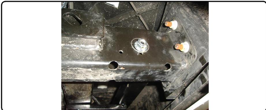
5. Install hex flange nuts onto carriage bolts fishwired in step 3.
