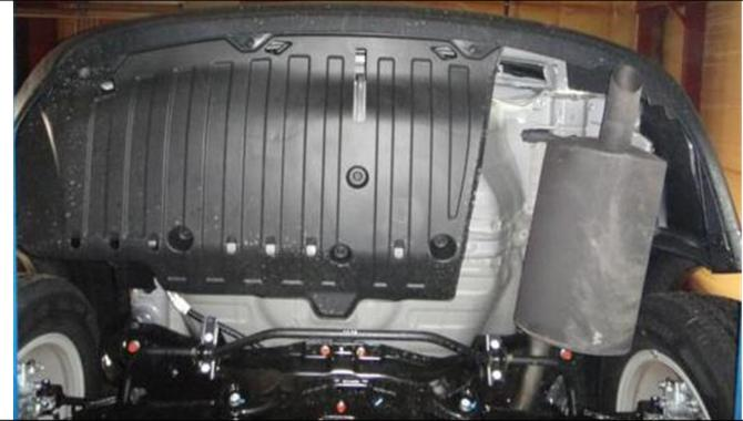
2. Lower exhaust by removing (2) rubber isolators from the hangers attached to the exhaust.
