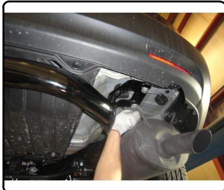
5. Torque all 7/16" hardware to 25 ft-lbs. Torque all 10mm hardware to 48 ft-lbs.
