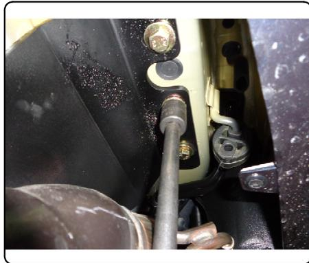
4.) Torque all M12 hardware to 86 ft-lb. Reattach all exhaust hangers.
