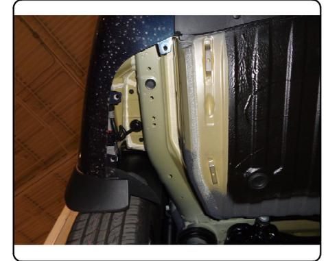
2.) Lower the exhaust by removing the (4) rearmost rubber isolators from the muffler hangers. Support exhaust from underneath.
