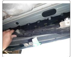
3. Remove rubber islolator brackets which are located to the inside of mufflers. Remove (2) bolts from each bracket and return bolts to vehicle owner.
