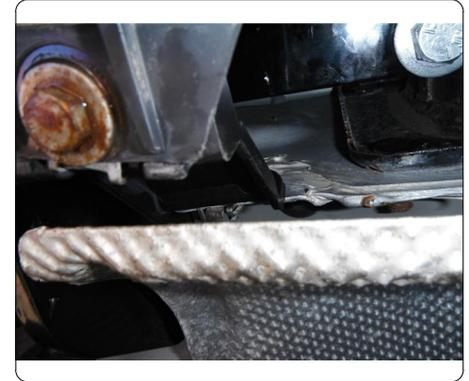
9. Raise exhaust back into position. **Note:** If heat shield contacts hitch, trim heat shield so there is 1/8" clearance. If exhaust tips were removed, reinstall with screws which were removed in step 1. Hitch installation is complete.
