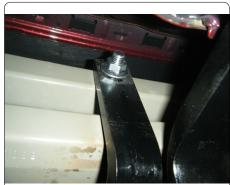
4. Fishwire 1/2" carriage bolts and CM-SP6 spacers into vehicle "A" frame and secure with 1/2" hex flange nuts.
