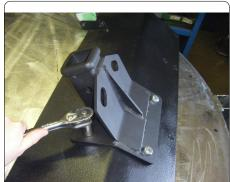
8. Reinstall vehicle skid plate. Torque factory M8 hardware to 23 ft-lbs.
