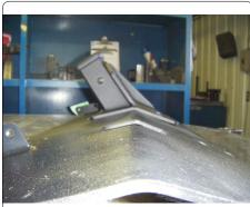
4. Mark locations of (4) holes and drill using a 9/16" drill bit. NOTE: Push drill through foam to show hole locations for STEP 5.
