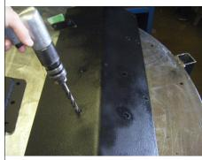
5. Trim foam on skid plate to allow clearance for 1/2" flange nuts at (4) mounting locations.
