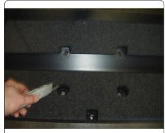
6. Attach hitch to vehicle skid plate using the included 1/2" hardware. (As shown in diagram on page 2.)
