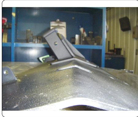
4. Mark locations of (4) holes and drill using a 9/16" drill bit. NOTE: Push drill through foam to show hole locations for STEP 5.
