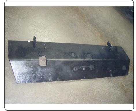
2. Mark center of vehicle skid plate which is at 24.125". (See CENTERING DIAGRAM below)
