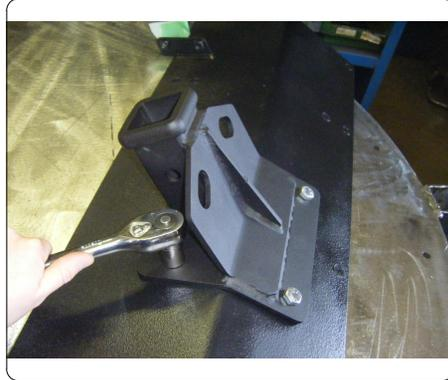
8. Reinstall vehicle skid plate. Torque factory M8 hardware to 23 ft-lbs.
