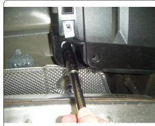
4. Pull down on rear fascia and remove fascia support brackets. The second photo shows the hardware removed. **Note:** Use masking tape to protect vehicle finish. Brackets will be reinstalled in Step 6.
