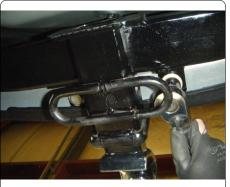
6. Reinstall fascia support brackets and fasteners. Torque all M12 fasteners to 79 ft-lbs.
