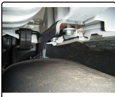
Re-attach (2) center rubber exhaust hangers which were removed in STEP 1.
