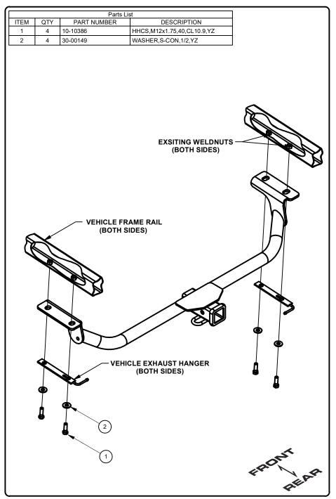
1. Remove (2) center rubber exhaust hangers. (See RUBBER ISOLATOR REMOVAL DIAGRAM) **Note:** Be sure to support exhaust so it does not bend in STEP 2.
