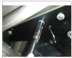
6) Raise exhaust into postion and secure isolator mounts using the bolts removed in step 3. Install is now complete.
