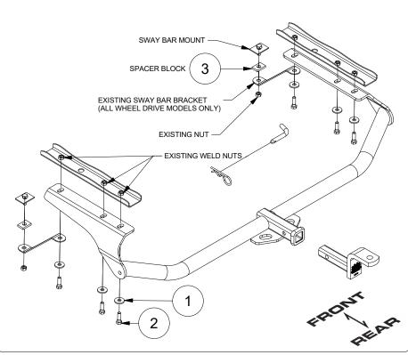
1) If the vehicle is all wheel drive, remove the (2) sway bar brackets. Save the existing nuts for use in step 4.
