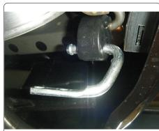
4) Raise the hitch into position and install (3) 10mm bolts and conical toothed washers per side into the existing weldnuts in the frame. If the vehicle is all wheel drive then reinstall the sway bar brackets using CM-SP50 spacer blocks and the existing nuts on the lower mounts.
