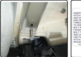
FISHWIRE TECHNIQUE INSERT COILED END OF FISHWIRE TOOL THROUGH HITCH MOUNTING HOLE IN VEHICLE FRAME RAI AND OUT THE ACCESS HOLE. PASS COILED END OF FISHWIRE THROUGH SPACER AND THREAD BOLT INTO COIL. KINK WIRE TO KEEP SPACER SEPERATE FROM BOLT AS SHOWN, PULL ACCESS HOLE FISHWIRE, SPACER, AND BOLT THROUGH FRAME AND OUT MOUNTING HOLE JSE FISHWIRE TO GUIDE ITCH DURING MOUNTING AND PREVENT LOSS OF BOLT / SPACER INSIDE FRAME RAIL \*NOTE: SOME VEHICLES MAY FISHWIRE THROUGH END OF FRAME
