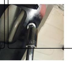
10. Center hitch on vehicle. Using the hitch as a template, drill front (2) holes in frame rails. Drill one hole per frame rail using a 17/32" drill bit
