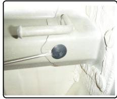
Enlarge front (2) holes where rubber plugs were removed in Step 6 with die grinder. Enlarge only enough to allow CM-SP6 spacers and 1/2" carriage bolts to pass through.
