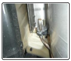
2. Remove (1) rubber isolator from exhaust tube forward of muffler.
