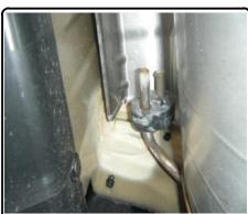
16. Reattach (1) rubber isolators on vehicle exhaust tube forward of muffler. Remove wire previously holding up exhaust.
