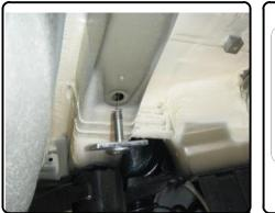
FISHWIRE TECHNIQUE INSERT COILED END OF FISHWIRE HITCH MOUNTING HOLE IN VEHICLE FRAME RAIL AND OUT THE ACCESS HOLE. PASS COILED END OF FISHWIRE THROUGH SPACER AND THREAD BOLT INTO COIL. KINK WIRE O KEEP SPACER SEPERATE FROM BOLT AS SHOWN. PULL ACCES FISHWIRE, SPACER, AND BOLT THROUGH FRAME AND OUT MOUNTING HOLE USE FISHWIRE TO GUIDE HITCH DURING MOUNTING AND PREVENT LOSS OF BOLT SPACER INSIDE FRAME RAIL \*NOTE: SOME VEHICLES MAY FISHWIRE THROUGH END OF FRAME\*
