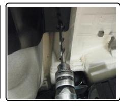
11. Fishwire 1/2" carriage bolts and CM-SP6 spacers through enlarged holes and out front mounting holes using supplied fishwire tools.
