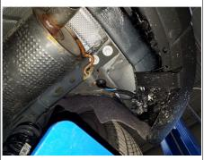
4. Feed the 1/2" handle nut through the access hole to the forwardmost attachment for the passenger sideplate. Attach the 1/2" hex bolt and conical tooth washer. Torque all M10 hardware to 45 ft-lbs. and all 1/2" hardware to 110 ft-lbs.
